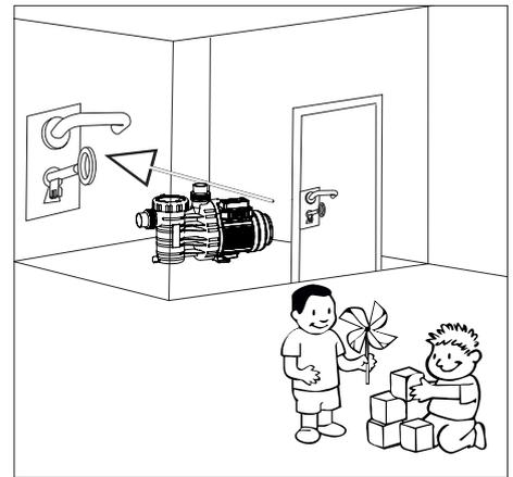
Ensure the motor's cooling. The installation site must be dry and well ventilated.
