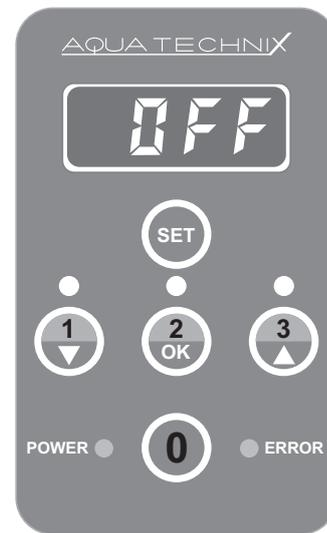
The display of the control unit switches off after 3 minutes without action.
